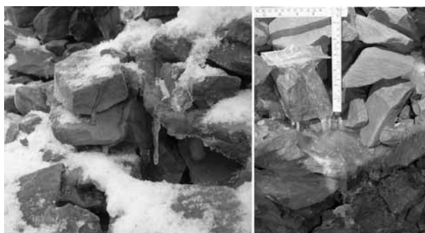
Figure 2. Photos showing icicles and interstitial ice in the pore volume of the active layer. Vertical section of ruler is 17 cm. Photos taken 26.04.2006 (left) and 04.05.2006 (right).
